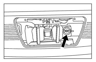
4. Reinstall the wing nut retainer to fasten the jack and tool bag in the storage compartment.
